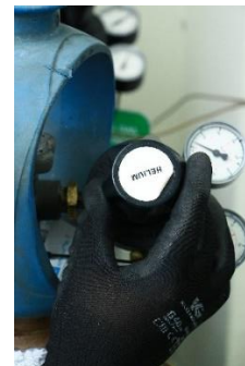
7. Ensure regulator pressure adjusting screw is closed.
