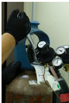
6. Use wrench to securely tighten regulator. Secure regulator tight enough not to leak.
