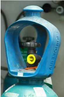
1. Inspect cylinder valve outlet from any damage
