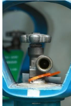
3. Inspect cylinder valve outlet for contamination. Momentarily open and close cylinder valve to clear any contamination that may be present. Do not vent the valve if handling Toxic or Poison gases. Avoid doing this practice with Hydrogen, it may explode.
