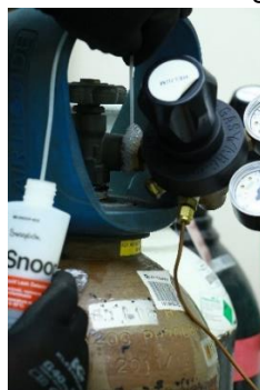
10. Spray or apply the soapy water solution onto the area you want to test, such as a joint or fitting, and watch for bubbles. The soap solution will bubble if there is a gas leak or other fault in the line.
