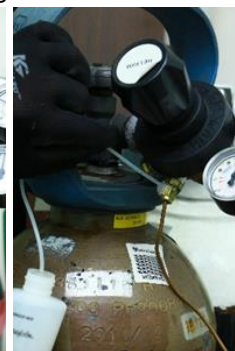
10. Spray or apply the soapy water solution onto the area you want to test, such as a joint or fitting, and watch for bubbles. The soap solution will bubble if there is a gas leak or other fault in the line.
