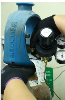
5. Attach regulator to cylinder valve
