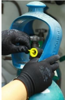
2. Open valve outlet sealed
