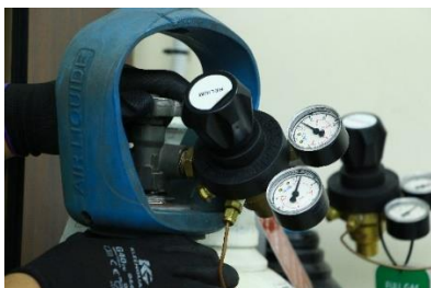
9. Open the cylinder valve slowly until pressure gauge is fully pressurized.
