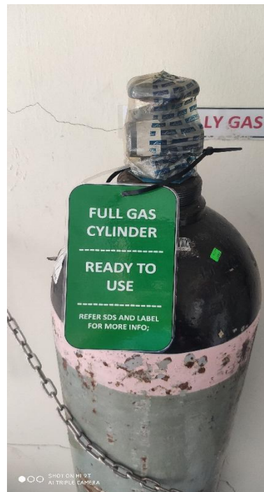
Picture 4: Label for full gas cylinder and ready to use
