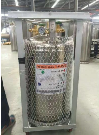
Picture 2: Example of mechanical support for transporting Liquid Nitrogen container.
